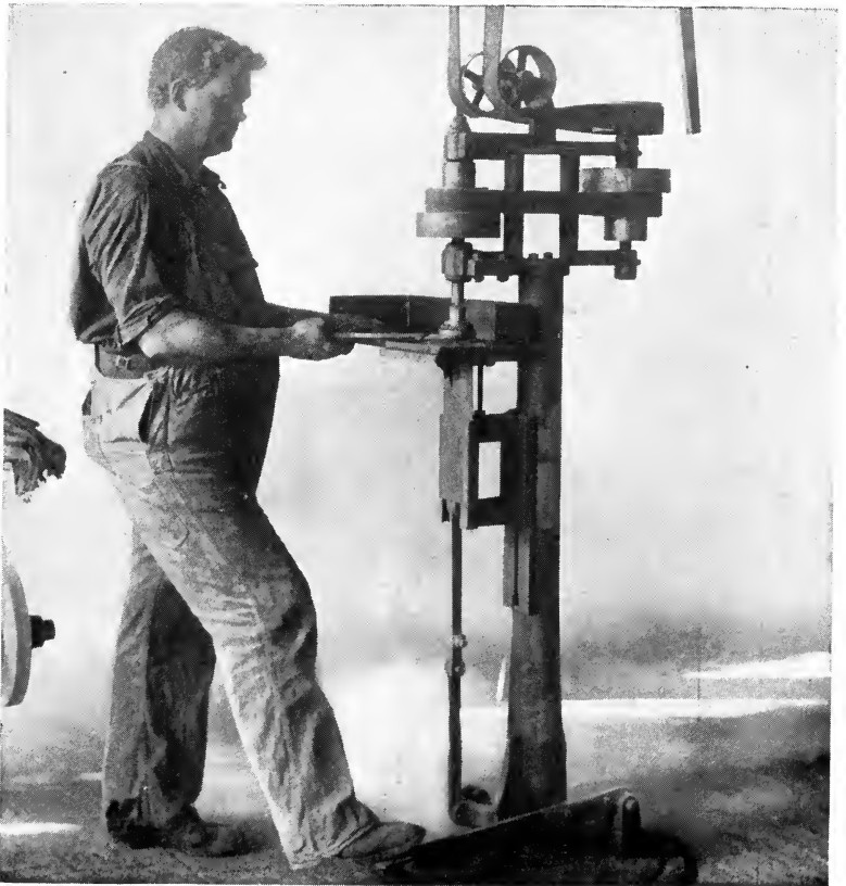
By standardizing operation, standardized material and labor costs become possible. In a steel plant the one best way (below), of polishing nickeled cups was found after the two methods shown at the left and right, above, had been discarded. Formerly, the polishing part of the machine was horizontal and operated by hand. By turning the machine "on end," output was increased 500%
